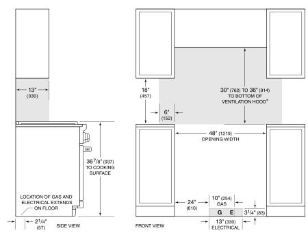
\*Without ventilation hood, 36" (914) minimum clearance countertop to combustible materials, 44" (118) for charbroiler. NOTE: Shaded area above countertop indicates minimum clearance to combustible surfaces,
