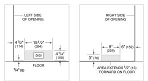
$\ensuremath{\text{NOTE:}}$  The electrical outlet must be positioned with the grounding prong to the right of the thinner blades.
