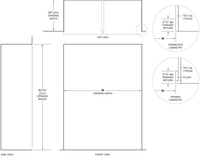
NOTE: 31/2" (89) finished returns will be visible and should be finished to match cabinetry. Shaded line represents profile of unit.
