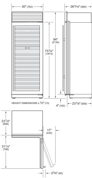
**IMPORTANT NOTE:** Overall dimensions are based on the stainless steel model. For flush inset applications, add  $\frac{1}{2}$ " (13) to door clearance dimensions.
