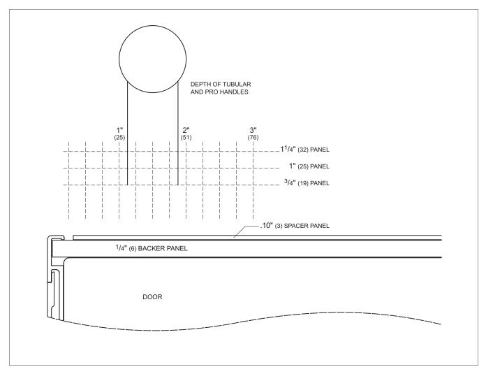
Overlay and flush inset panel thickness
